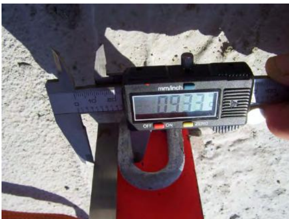
PHOTO 3: EMBED LOOP PRIOR TO TESTING (0.933 in)
