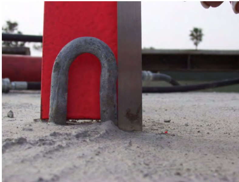
PHOTO 5: DEFORMATION OF EMBED LOOP
