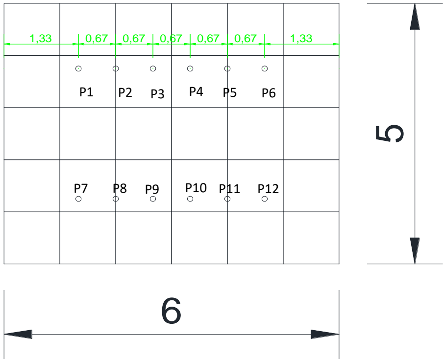
Load to panel based on Bar Mat Capacity per Bar Mat Point
