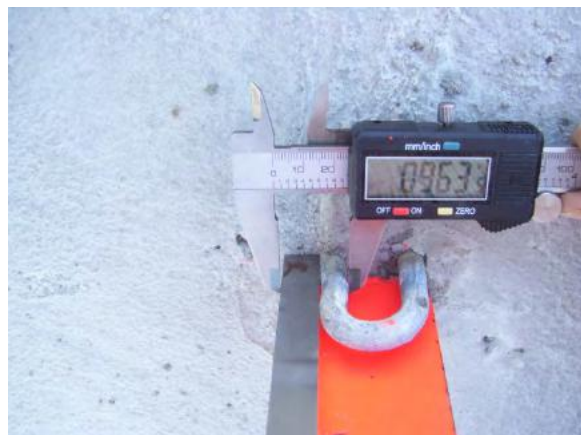
PHOTO 4: EMBED LOOP AFTER W20 TEST (0.963 in)
