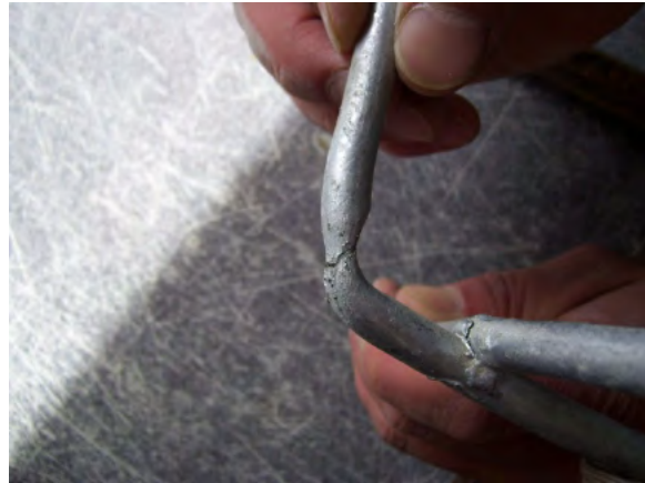
PHOTO 2: W11 NECKED DOWN AND FRACTURED
