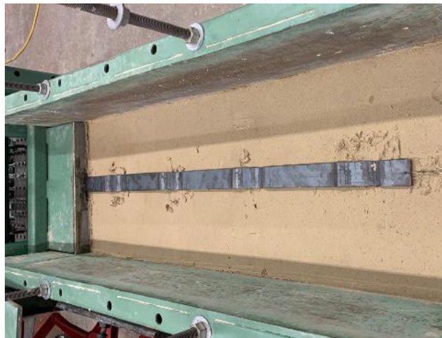
Photograph 2-5 LVDT Location Attached to Soil Reinforcing Inside Soil Box
