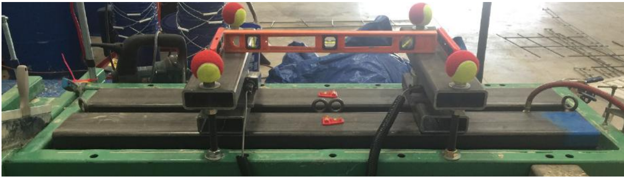
Photograph 2-2 Vertical Overburden Apparatus
