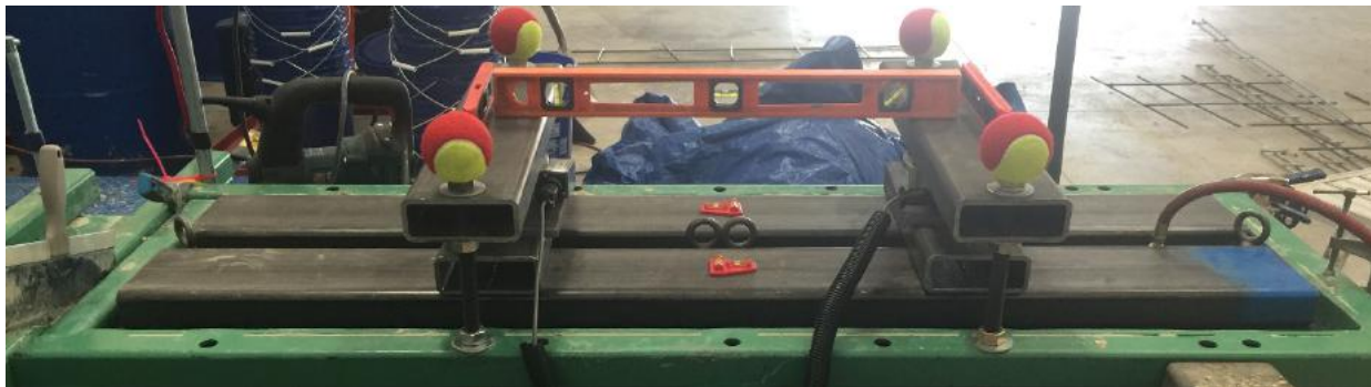
Photograph 2-2 Vertical Overburden Apparatus with Structural Steel Reaction Frame
