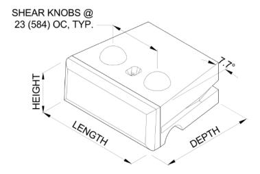
Figure 7 - Block dimensions
