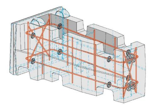
Fig. 2. Reinforcement cage for Redi-Rock XL units.
