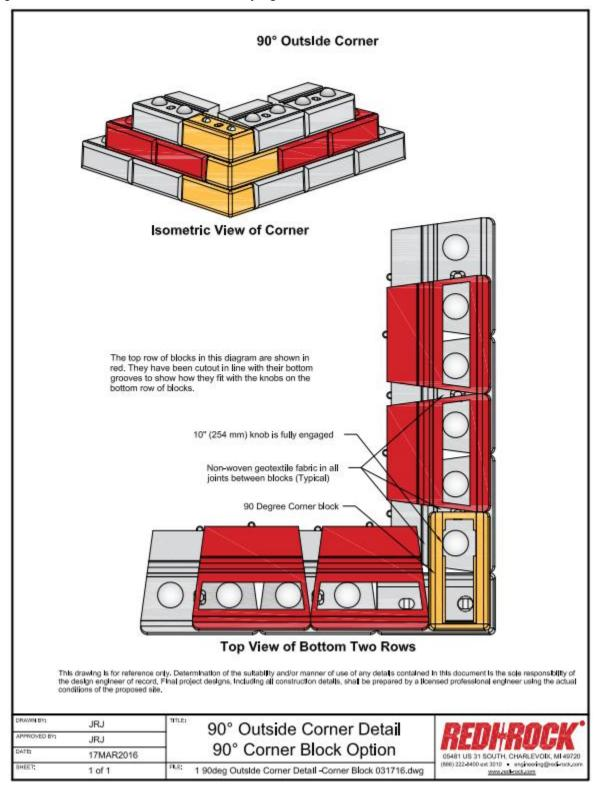
Figure 29 - Outside corner detail
