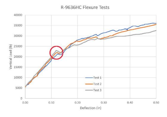
Fig. 15. Close-up view of the load-deflection curves at first yield.
