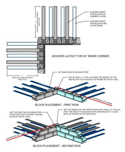
Figure 38 - Geogrid layout for 90° inside corner
