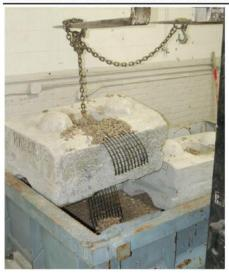
Figure 6 - Exhuming Geogrid from Block
