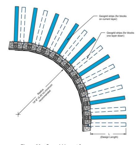
Figure 36 - Geogrid layout for concave curves
