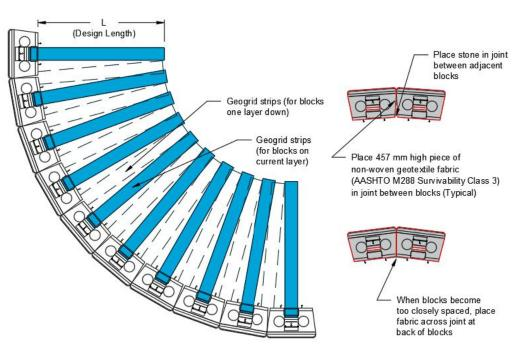
Figure 37 - Geogrid layout for convex curves
