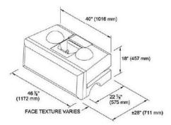
Figure 2 - PC Block Dimensions
