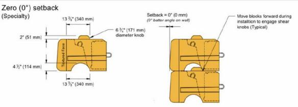
Figure 13 - Standard block face batter options
