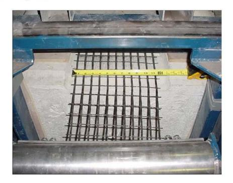
Figure 3: Photograph of the Redi-Rock Positive Connection (PC)
