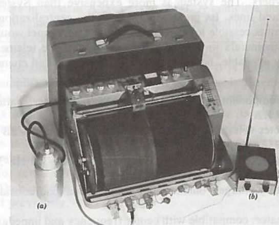
FIG. 3.—Single Sensitive Station of System A (Portable Seismograph Records on Smoked Paper and Contains Its Own Batteries): (a) Seismometer; (b) Radio Receiver
