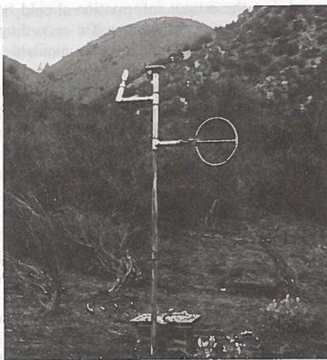
FIG. 2.—Unattended Field Installation of Strong Motion Accelerograph [Vertical Pole Supports Circular Loop Antenna for Time Signals (Right) and Two Solar Cells for Charging Batteries; Protective Housing Contains SMA-1 Accelerograph; Radio Receiver; and Power Batteries Supply; and Pole (approx 3m high)]
